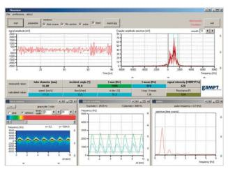
or the investigation of the pulsatility of the flow. By limiting the measurements to particular times of flight (sample volume) it is possible to gain information from limited areas of the tube cross section and thus different layers of the flow. In this way a velocity profile and a concentration profile of the flow can be produced.
