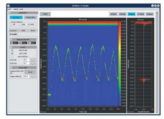
IND07 Crack depth determination (TOFD)
