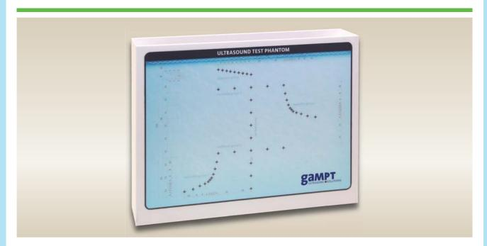
Tissue-equivalent phantoms are used for quality assurance and evaluation of the accuracy and performance of imaging ultrasonic systems. The phantoms are made of materials possessing physical characteristics similar to the acoustic characteristics of human tissue.
