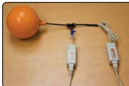
Accessory kit being used with a ball cock, Pressure and Temperature sensor to investigate Charles Law.
