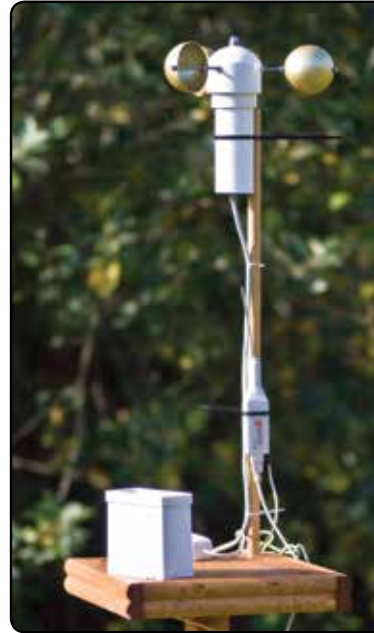
An improvised weather station using the Count Tachometer with the Rain Gauge and Anemometer connected to a data logger for long term recording.
