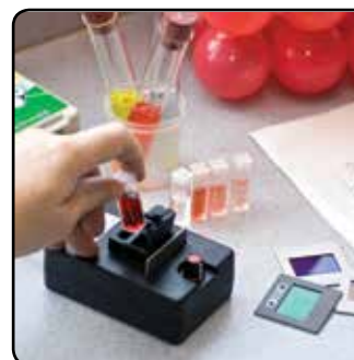
The sensor's thick, black casing ensures that colorimetric results are not affected by ambient light.
