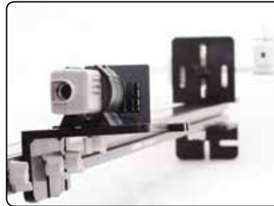
Laser mounted on the Dynamics System investigating diffraction patterns.
