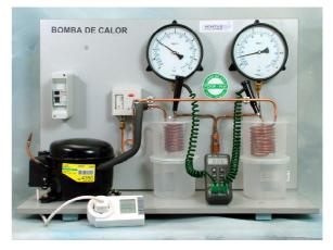
Determining the efficiency of the heat pump as a function of the temperature differential (Not included: Power and temperature meter, ask for quotation).
