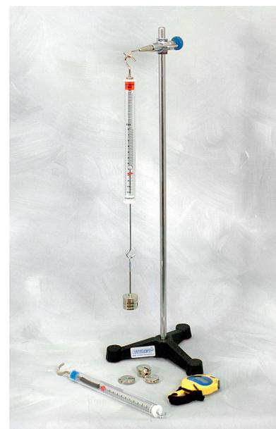
Example of arrangement for Hooke's Law and harmonic oscillations.
